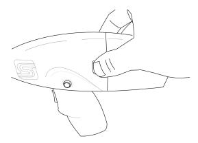
3. If the device is mid-fire, the knife can be manually reset (i.e. brought back to the starting position) by inserting the Bailout Key into the bottom (black) gear.
